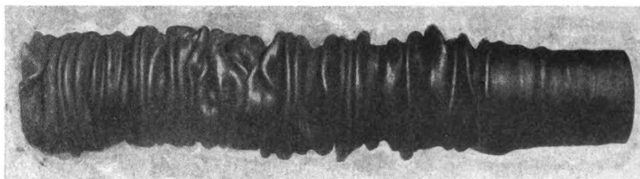
Shelby Steel Tube Upset at Both Ends, Showing Quality.
